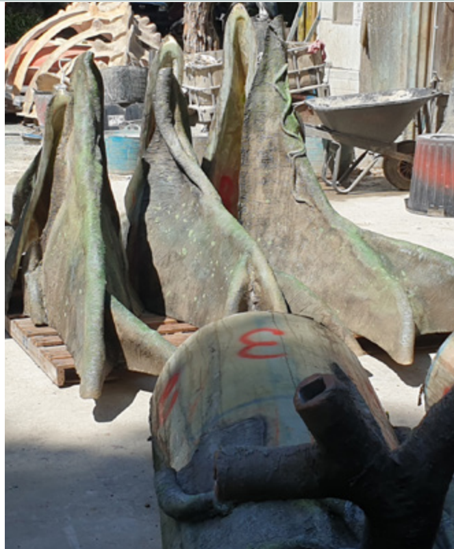
The tree was made in six pieces for easier transport and installation
