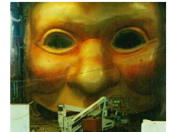
Step 3. Creating a heavy duty fibreglass shell over the sculpture; removing the polystyrene and applying colour/texture.
